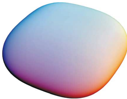
Fig. 20. Tetragonal system: material belonging to Class 2b, defined in Table 4. \text{Pb}_{0.37}\text{Ba}_{0.63}\text{Nb}_2\text{O}_6 (lead barium niobate): A' = 1.66 , B' = 1.28 and C' = 0.78 (dimensionless); \alpha_2 = -3.8 , \beta_2 = -3.2 , \beta_3 = 2.6 (expressed in \text{TPa}^{-1} ); Elastic compliance coefficients (taken from Landolt and Börnstein, 1992 and expressed in \text{TPa}^{-1} ): s_{11} = 5.80 , s_{33} = 9.60 , s_{44} = 18.20 , s_{66} = 12.40 , s_{12} = -1.70 , s_{13} = -1.70 . Young's moduli (in GPa): E_{\min} = .104167 and E_{\max} = .194175 .
