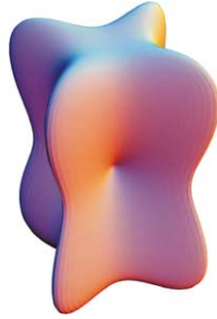
Fig. 11. Tetragonal system: material belonging to Class 1d, defined in Table 4. (\text{NH}_2)_2\text{CO} (urea): A' = 0.67 , B' = 0.32 and C' = 11.86 (dimensionless); \alpha_2 = 31.0 , \beta_2 = 130.0 , \beta_3 = -2062.0 (expressed in \text{TPa}^{-1} ). Elastic compliance coefficients (taken from Landolt and Börnstein, 1992 and expressed in \text{TPa}^{-1} ): s_{11} = 95.10 , s_{33} = 64.00 , s_{44} = 160.00 , s_{66} = 2220.00 , s_{12} = 16.00 , s_{13} = -50.00 . Young's moduli (in GPa): E_{\min} = .001638 and E_{\max} = .019112 .
